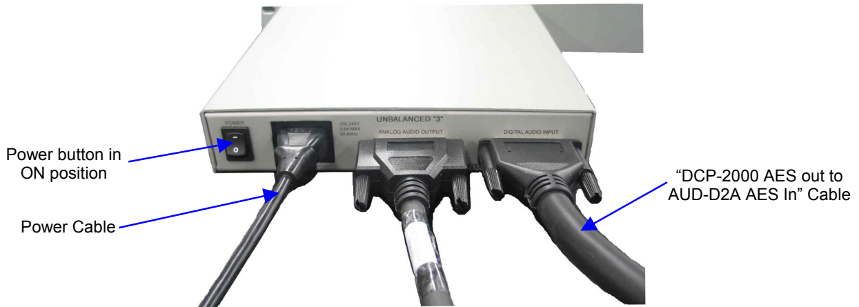
Figure 9: AUD-D2A Rear Panel – AES Cable Connection
