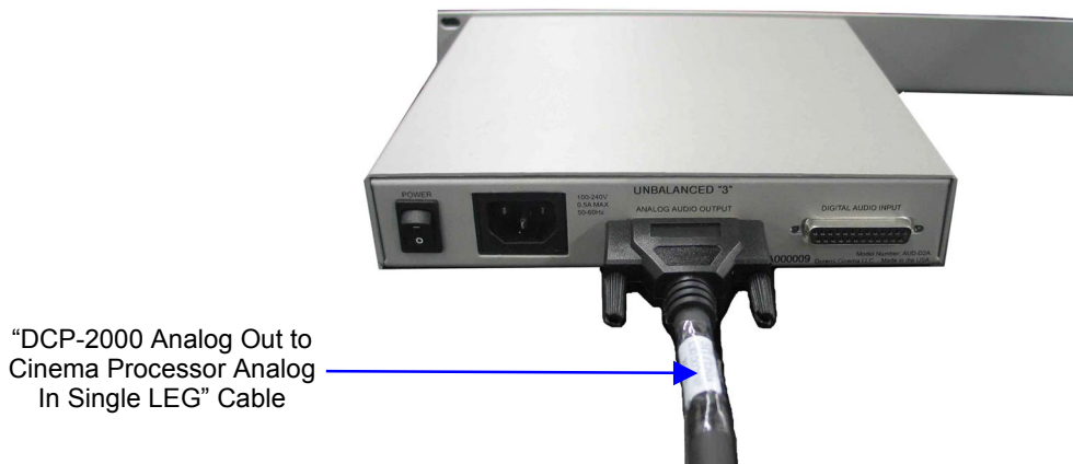
Figure 6: AUD-D2A Rear Panel – DCP-2000 Analog Cable Connection
